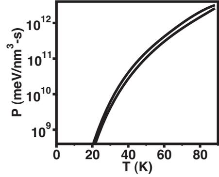
FIG. 6. Calculated energy transfer rate in  $\text{meV}/\text{nm}^3 \text{ s}$  of electron gas at temperature  $T$  to a zero-temperature lattice. The lower curve represents the phonon emission process and the upper curve represents the quasiparticle annihilation process.
