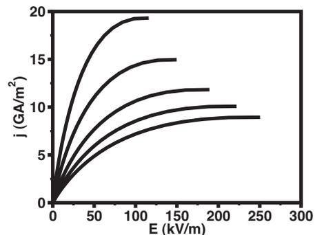
FIG. 1. Effect of increasing flux density on the current density vs electric field curve calculated in the model with variable  $\tau_\epsilon$ . Values of  $B$  beginning at the upper curve are 3, 5, 8, 11, and 14 T.
