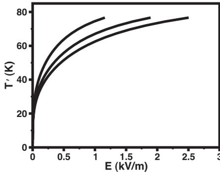
FIG. 3. Calculated electron temperature  $T'$  vs electric field  $E$  for  $B=3, 8,$  and  $14$  T, with  $B$  increasing from left to right.
