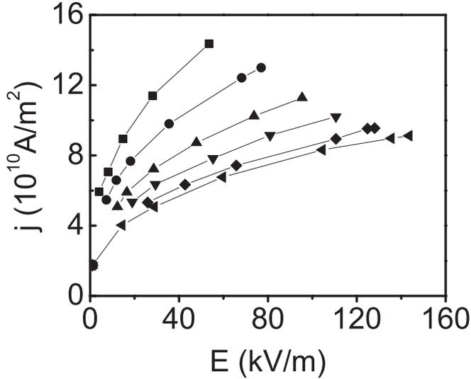
FIG. 2. Experimental curves of current density vs electric field in YBCO for flux density (beginning with the upper curve)  $B=3, 5, 8, 11, 14,$  and  $16$  T.
