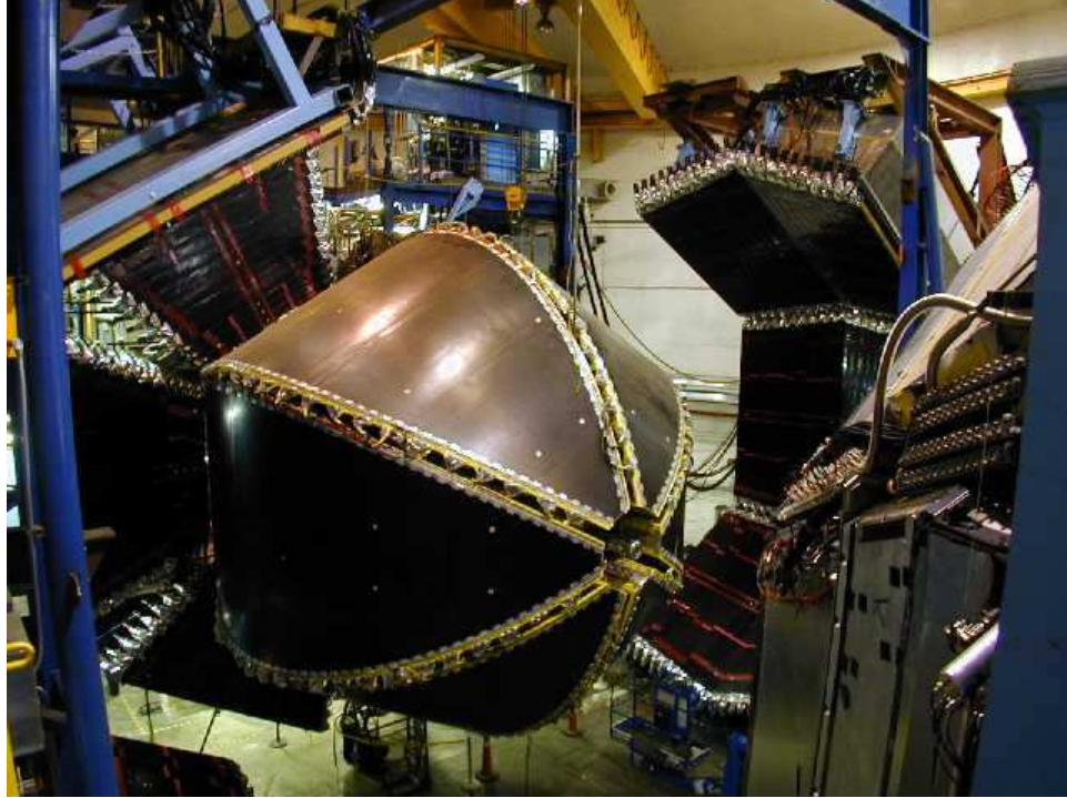
FIGURE 2.4. A picture of CLAS. The drift chamber detectors (DC) are still closed inside, and the time-of-flight detectors (TOF) are opened up and peeled away.
