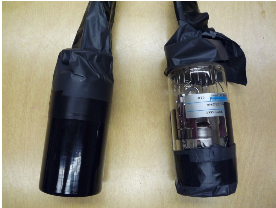
Figure 14: PMT with mu-metal shielding (left) and without shielding (right) 15 .
