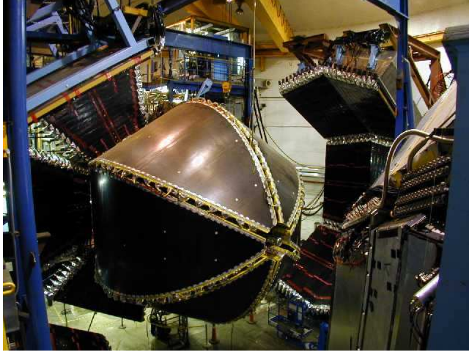
FIGURE 2.6. A picture of the CLAS. Inside you can see is the drift chamber (DC), and the black peeled away is the time-of-flight detector (TOF).
