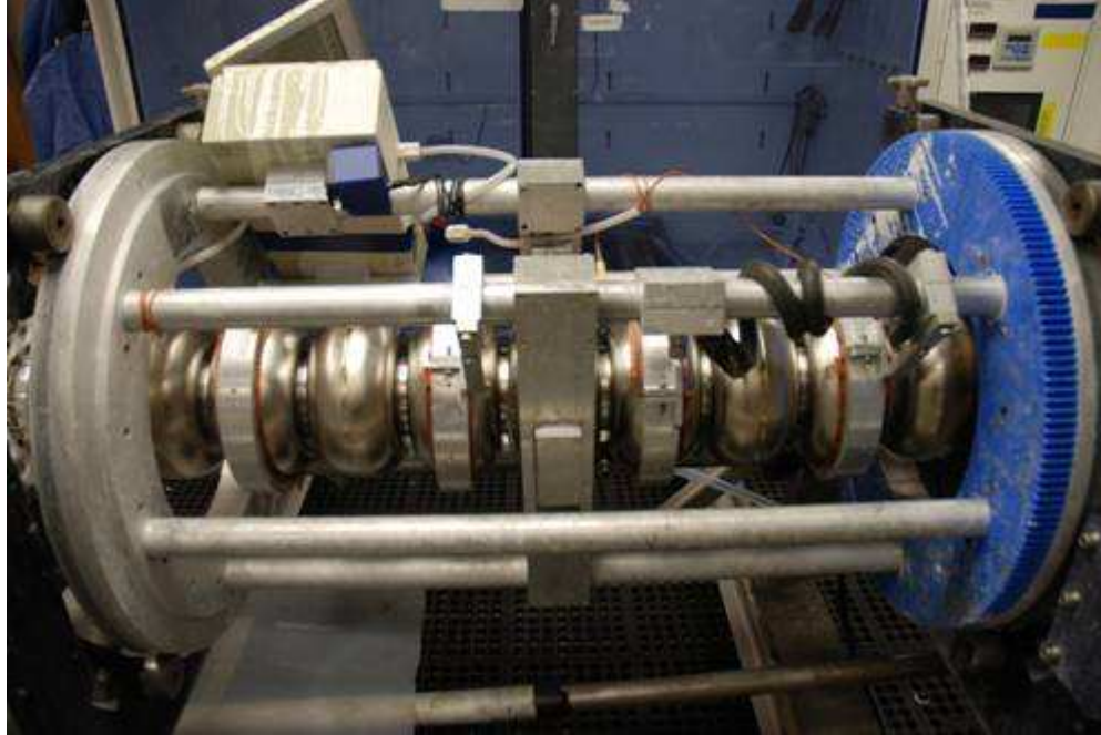
FIGURE 2.3. Picture of CEBAF's SRF cavities.
