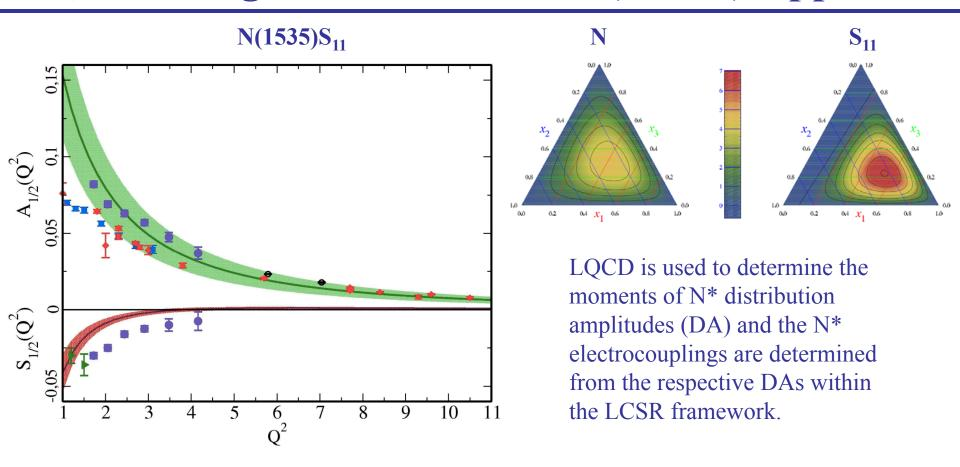
Calculations of  $N(1535)S_{11}$  electrocouplings at  $Q^2$  up to 12 GeV<sup>2</sup> are already available and shown by shadowed bands on the plot.
